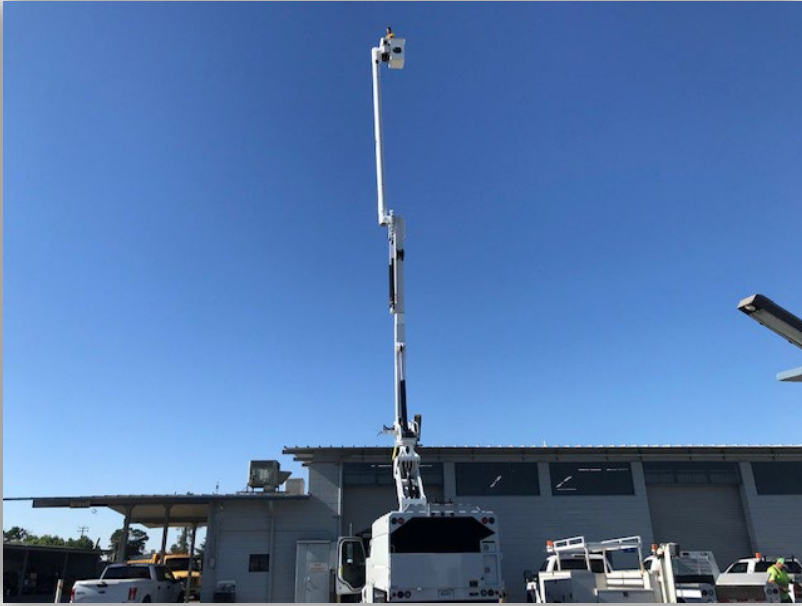
Streets Division checking the operation of the new aerial truck that can reach a height of 70 feet.
