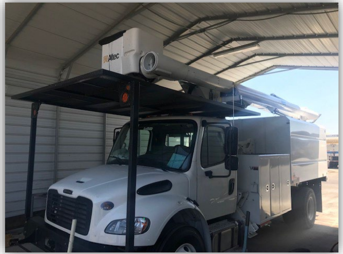
Streets Division checking the operation of the new aerial truck that can reach a height of 70 feet.
