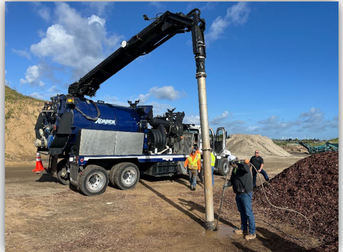
Water Department crews attended a demo for a hydrovac truck.
