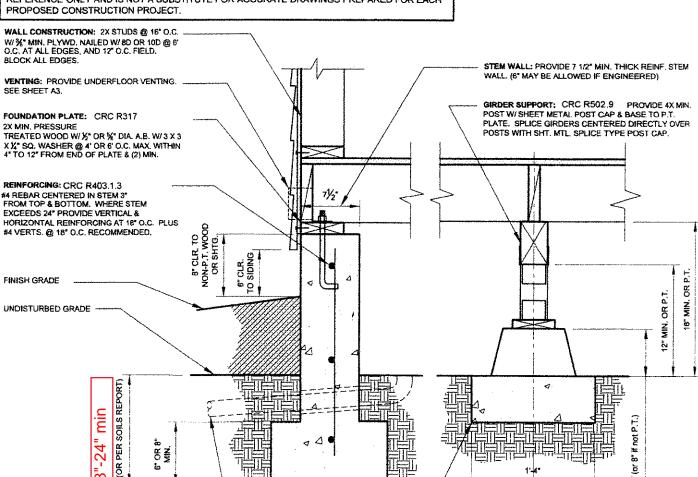
UNDERFLOOR DRAINAGE: CRC R405 PROVIDE UNDERFLOOR DRAINAGE WHERE UNDERFLOOR GRADE IS BELOW ADJACENT EXTERIOR GRADE.
