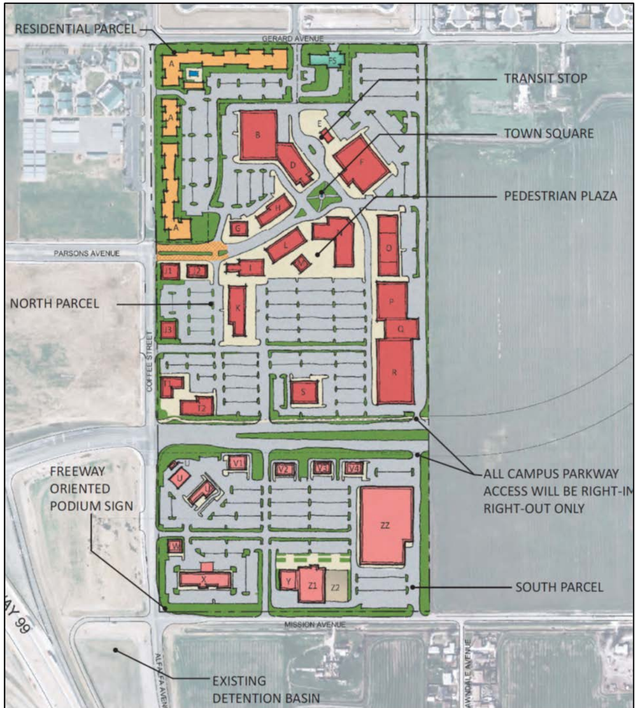
Figure 2 Conceptual site plan for the Merced Gateway Project, City of Merced, California.
