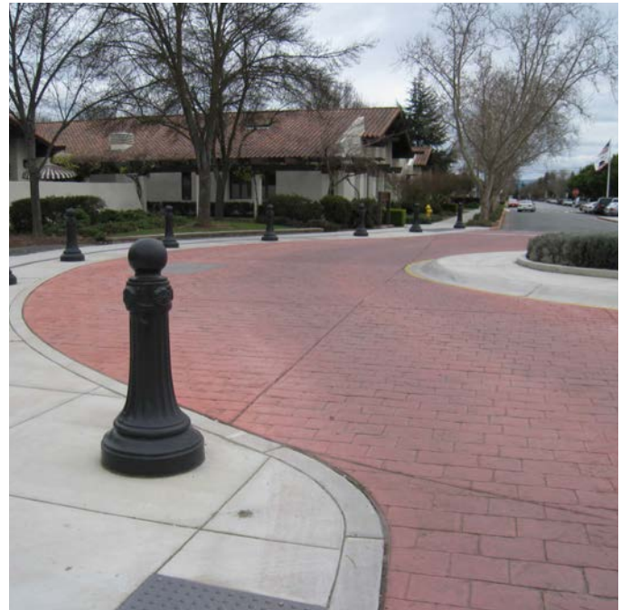
Passenger drop off area designated with special paving
